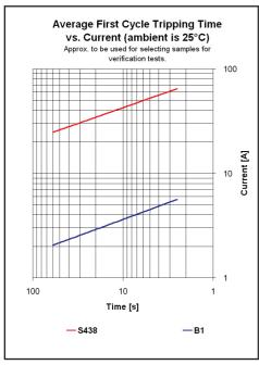
The curves of First Cycle Tripping time and Ultimate trip current are meant to be for selecting samples to perform verification tests only. In the figures two curves of a wide range of possibilities are shown. The level and slope can be varied by making an other selection for the pre-set temperature, bimetal disc and/or heater.
